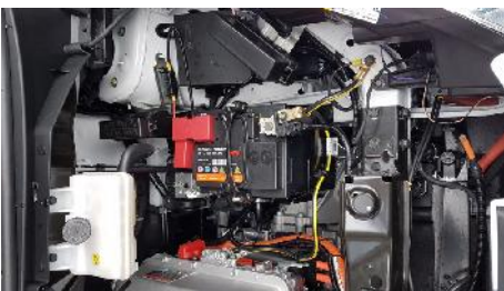
System battery and electric motor
