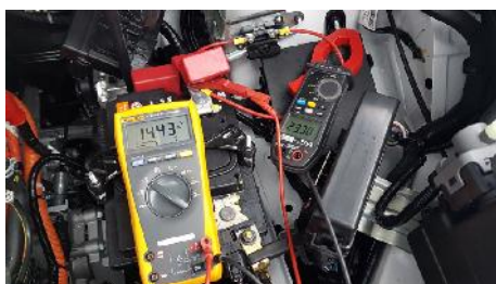
DBM charging current (23A) and System battery voltage 14.4V
