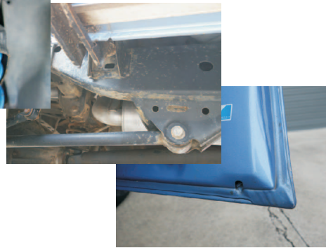
no rust at door rabbet (always rusting)
